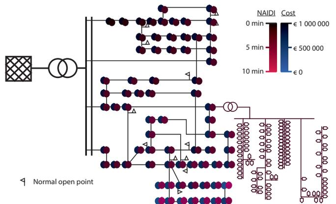
Fig. 4. Maximum change in NAIDI at each node and the associated costs for the conventional method of adding more MV-cables
