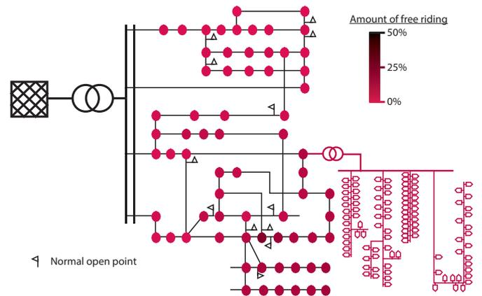
Fig. 6. Percentage of free riding due to the implementation of remotely-controlled switches
