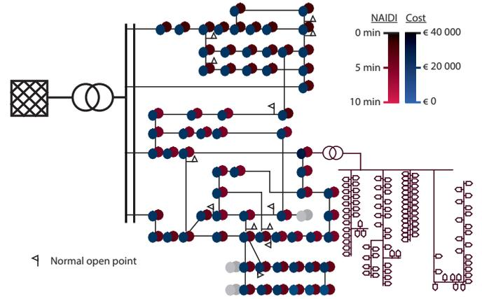
Fig. 5. Maximum change in NAIDI at each node and the associated costs for placing remote controllable switches
