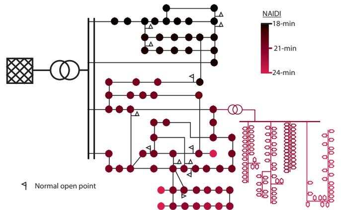
Fig. 3. Nodal average interruption duration index without the addition of smart grid technologies
