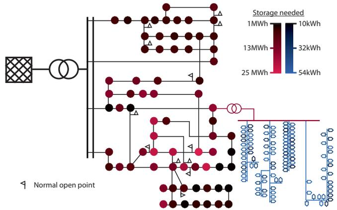
Fig. 7. Required storage need to mitigate the impact of outages on the MV and HV level
